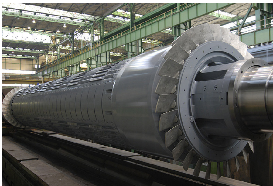
Fig. 8. Rotor of TWW-320-2Y3 generator with modernized fans with blade angle setting.
